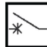
Figure 3 – Disconnecting circuit breaker
