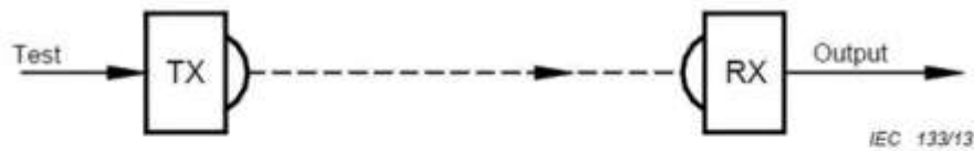
Figure AA.1 – Single beam sensing device
